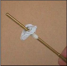
A special tool (M-260) is used to set the pedestals. It holds the pedestal as the epoxy is applied, and protects the opening into the void from oozing epoxy that may otherwise clog it. The M-260 Setting Tool also guides the pedestal to its precise location.
