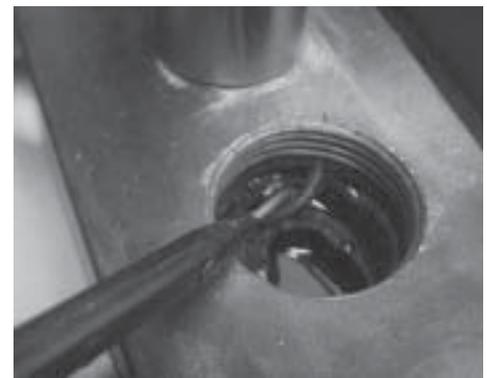
6. Lubricate the threads of the replacement metering assembly with an anti-seize compound or silicone lubricant. Thread the assembly into the manifold by turning it clockwise until it is seated. Do not overtighten. As the chamber bottoms out in the manifold you will feel a definite stop. Do not tighten further.
