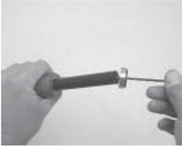
9. If the piston cap is larger than the piston diameter, it, and its pad, must be removed to insert the piston back into the cylinder.
