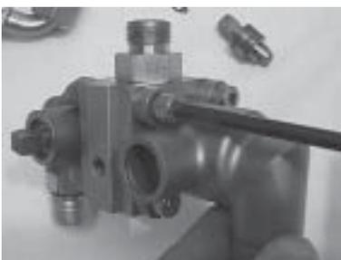
9. Attach the valve body to the block. Take care not to distort the o ring seal. Snug, but **do not tighten, the bolts until step 16!**
