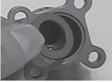
1. Fit the seal spring (S-330) into the pocket with its concave side toward the ball.
