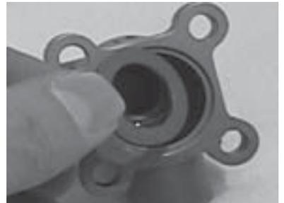
**Cleaning** Clean the components thoroughly, but do not use steel bristle brushes or instruments likely to scratch or gouge. Most solvents and cleaning agents can be used without damage to the stainless steel parts.
