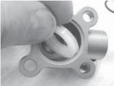
3. Insert the seal perpendicular to the bore until it is within the pocket. Then, twist it flat so that the spring side of the seal is facing down.
