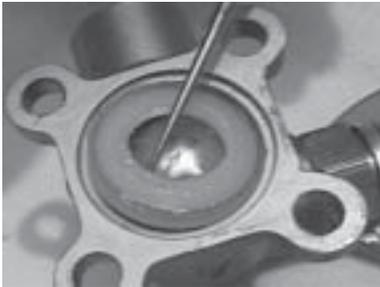
9. Use a seal pick to remove the seal (S-332). Take care not to scratch the ball or the wall of the pocket.
