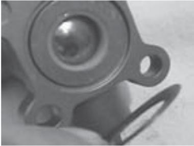
7. Remove the O-Ring (S-509) and the seal spring (S-330) (concave washer).
