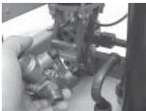
3. Pull the assembly from the frame. If it is not free, use a plastic, wood, or rubber instrument to urge it loose.
