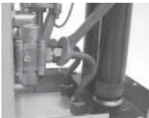
1. Use a 15/16” wrench to loosen the zero clearance fittings at the rigid tube segment (M-617). Remove the tube, taking care not to lose the seals within the fittings.
