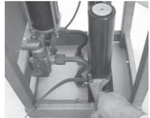
5. Use the seal pick to remove the base manifold o-ring. Clean the pocket thoroughly, and install a new o-ring in the lower groove.
