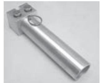
There are two types of shut-off valves to serve different applications. The Twin Shut Off valve (TSO) controls the flow of components dispensed through twin hoses. The components are not joined until within an inexpensive static mixer. The Single Shut Off (SSO) dispenses joined components from a single hose. SSO dispensing requires the use of a Gusto pump tank for cleaning.
