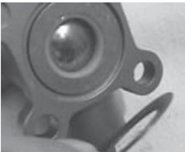
7. Install the flat washer over the seal, and apply silicone lube to hold it in place. Install the spring, concave side to the ball!!
