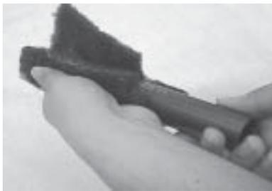
5. If the piston is scratched or marred, polish its surface with an abrasive cloth until no burr remains to damage the metering sleeve.
