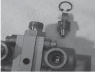
5. Grasp the coupler shaft (M-581) with a cushioned tool, and gently work it and its bushing (M-802) from the cavity.
