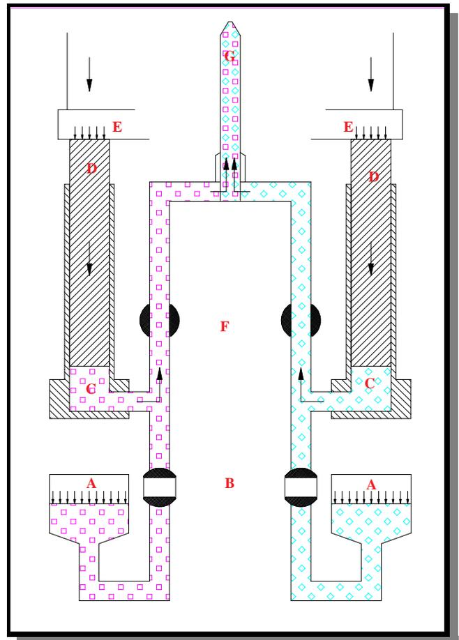
The resin components are pressurized within vessels (A) or by pumps. Pressurized, the components flow through open inlet valves (B) to enter their respective metering cylinders (C).
