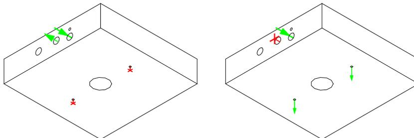
The vents are sealed off by the impingement of the ends of both of the metering pistons when fully extended. Once both of the vent holes are sealed, (confirming the arrival of both pistons) air pressure can then build to trigger the dispense cycle.
