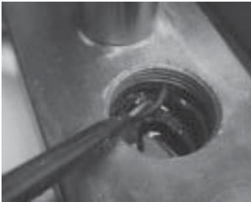
11. Use the seal pick (P-457) to remove the base manifold o-ring seal. Clean the pocket thoroughly before installing a new seal.
