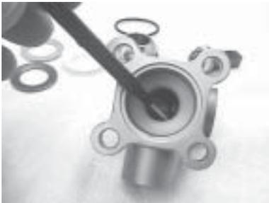
11. Use the seal pick to gently urge the lower seal from its seat. Take care not to scratch the housing.
