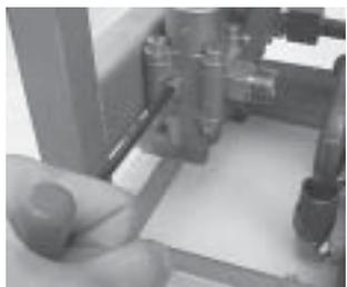
15. Secure the valve assembly to its frame. Apply an anti-seize compound to the threads of the mounting screw (S-334).
