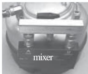
3. Disconnect the mixer or hose manifold block from the fluid outlet fittings and cap them with the caps secured at the magnetic bracket. Then secure the mixer or manifold block to the adapter block at the Gusto Purge tank. Make certain the fluid valves are closed. Disconnect the air supply from the dispenser, and connect it at the Gusto Purge air inlet. Rotate the selector valve to point to the mixer or hose manifold.
