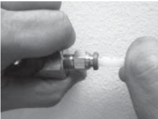
The air fittings are the 'press-to-connect' variety. The connection is made by firmly inserting the nylon tubing end into the fitting. The tubing is released by pulling the fitting collar firmly back against the fitting body, while pulling the tube from the fitting.
