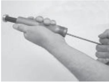
3. Press the metering piston from the cylinder bore. If it is seized, phone Lily or visit a machine shop for assistance. Do not damage the bore!
