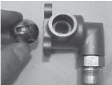
5. Slide the ball into the pocket with the detent (slot) facing the coupler pocket. Use the tang of the coupler shaft (M-581) to squarely align the ball slot.
