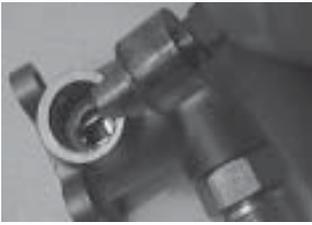
11. Carefully insert the coupler shaft (M-581), bronze bushing (M-802) and washer (P-469) into the housing.
