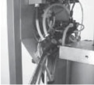
Periodic (twice a year) lubrication of the pneumatic components is recommended. To do so, de-energize the system and remove the right-hand -cover. Use a 9/16” open-end wrench to free the twin tube swivel compression fitting (P-093). It is not necessary to disconnect any tubing as the fitting body will swivel on its hex. .
