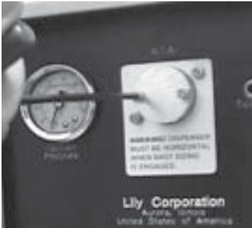
To connect the umbilical, remove the cap located on the front of the machine. Take care not to lose the o ring seals beneath the cap.
