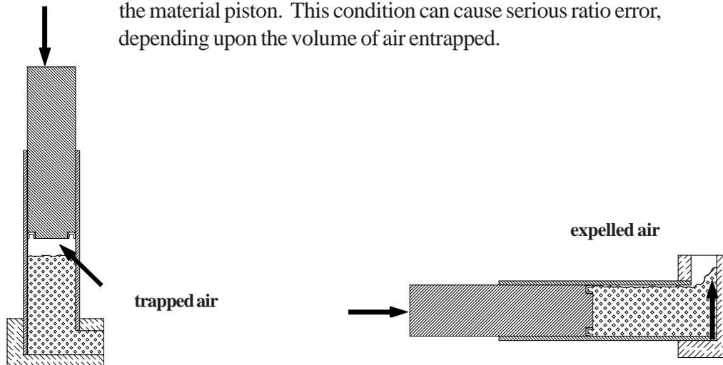
When the unit is horizontal, any air that enters the metering chamber is promptly expelled before it can accumulate to adversely affect ratio. .
