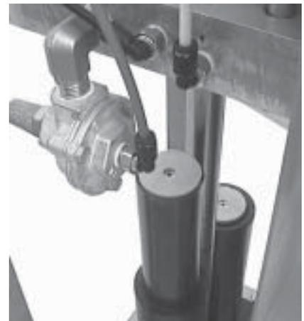
The metering pistons extend under fluid pressure
